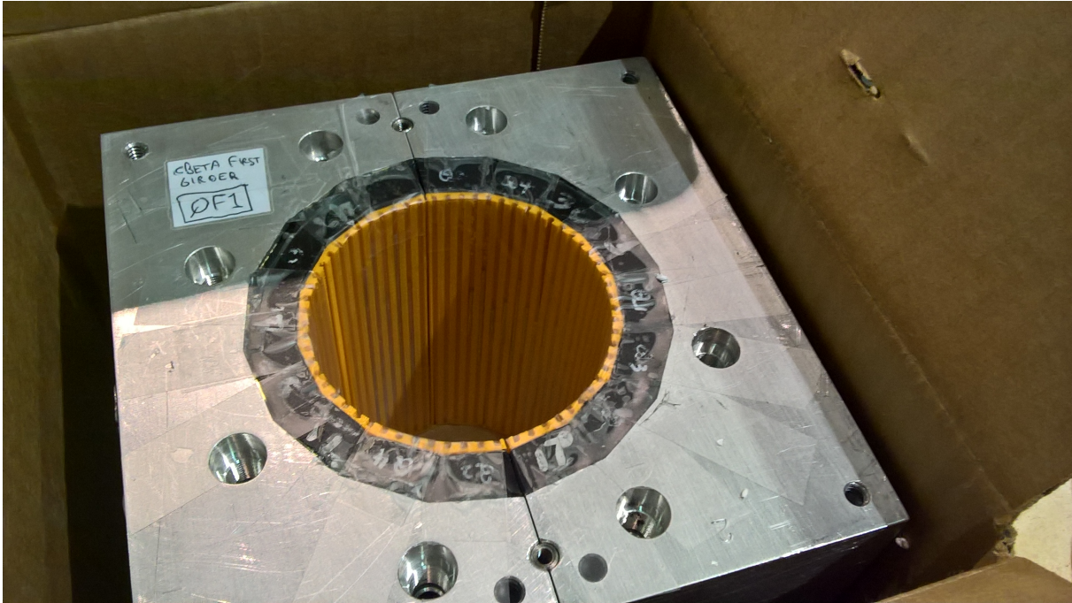
Figure 4: Iron wires were placed inside the QF1 magnet bore in order to cancel out field imperfections (“multipoles”). This photos shows them inside the orange 3D printed shim holder.
