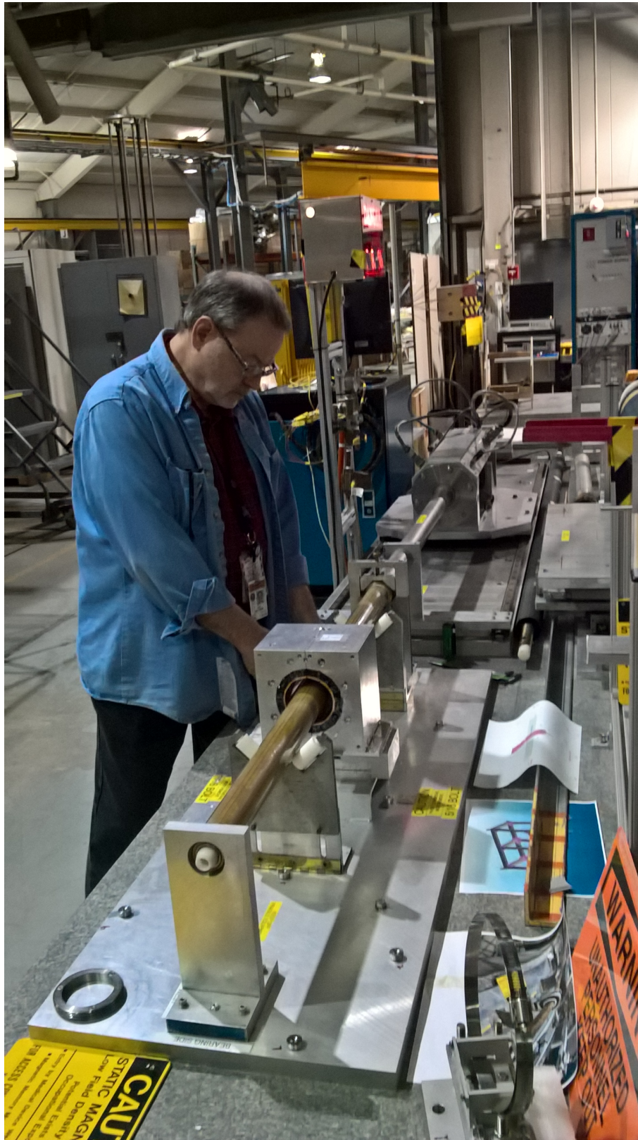
Figure 3: John Cintorino operates BNL's rotating coil apparatus for measuring multipoles in one of the girder's QF magnets (bottom center).
