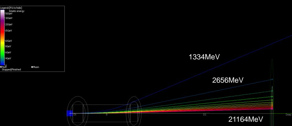
2m 0.92T dipole with -5T/m gradient Higher energies move into lower (and even negative) field region
